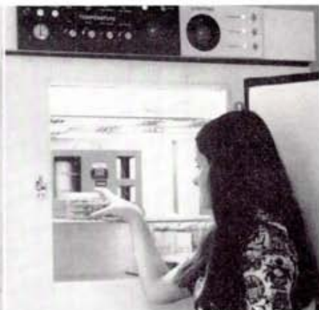
FIGURE 2. Percival growth chamber in which controlled studies are made of a strain of the fungus Glomerella cingulata pathogenic to camellias.
